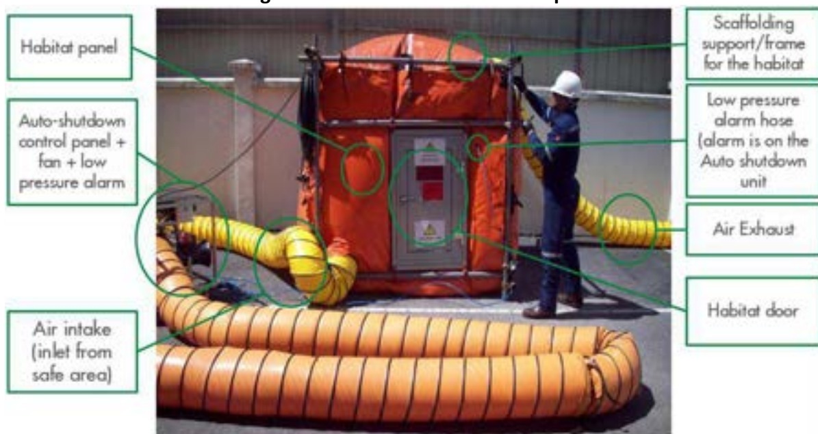
Figure 2 Pressurized Habitat Example
