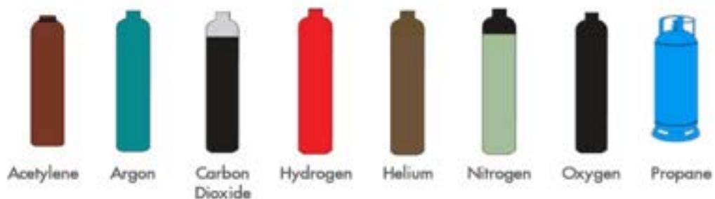
Figure 2 Industrial Gas Cylinder Colours
