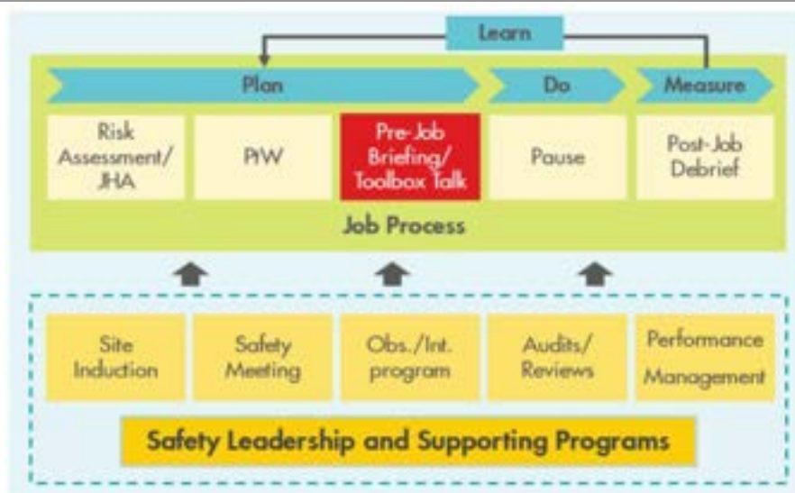
Figure 2 Worksite Hazard Management
